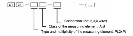
Example: Temperature sensor with transmitter, measuring range 0...60°C, Pt 100 sensor type, B class, 2 wires connection line.
